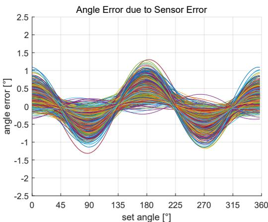
Figure 12: Angle error due to simulated sensor errors
