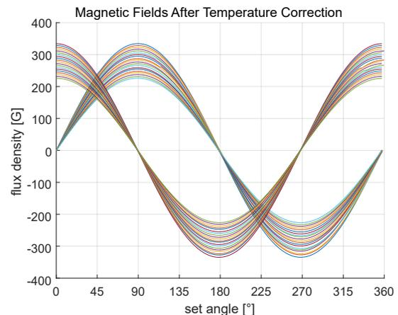
Figure 10: Temperature corrected magnetic field
