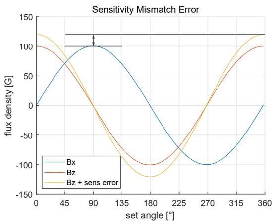
Figure 3: Example Channel Sensitivity Mismatch Error
