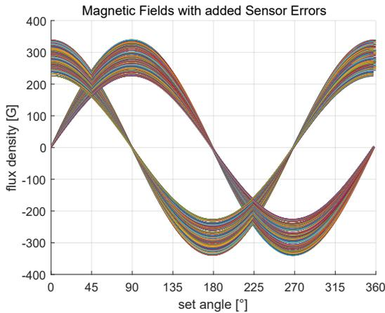
Figure 11: Temperature corrected magnetic field with added sensor errors
