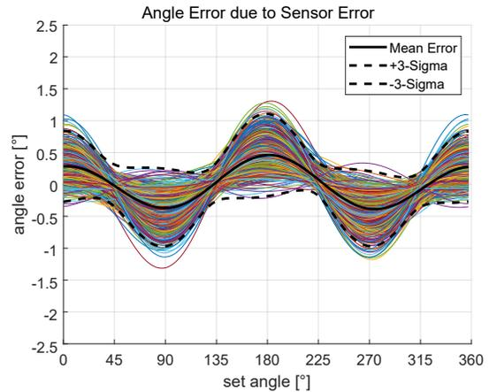
Figure 13: Angle error with calculated mean and sigma lines
