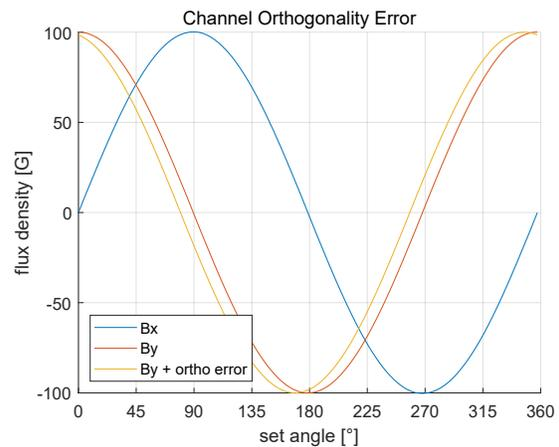
Figure 4: Example Channel Orthogonality Error
