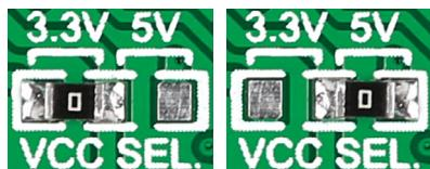
RTC4 click has a VCC SEL. jumper [zero ohm resistor] that lets you switch the board from **3.3V to 5V power supply**.
